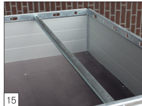
Option: load-restraint tubing mounted.
