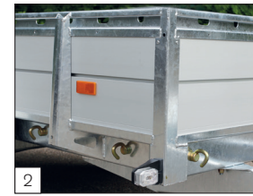
Option: boltable hooks on the outside.
