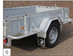
Option: protective brackets in front of, over, and behind the mudguards (from one piece) and provided with aluminium footboard. Mudguards of durable tread plate.
