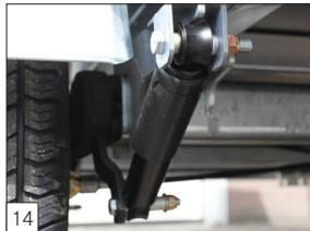
Option: shock absorbers mounted on axles.
