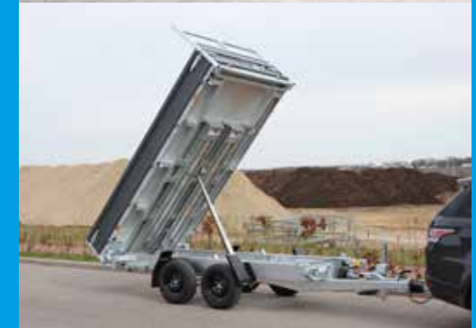
Standard: reinforced aluminium loading skids with a length of 2500 mm, integrated underneath the floor.
