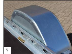
**Standard:** the mudguards have been closed on the inside. Provided with TÜV-certified binding brackets, integrated in the side rail, with a capacity of 1000 daN each.
