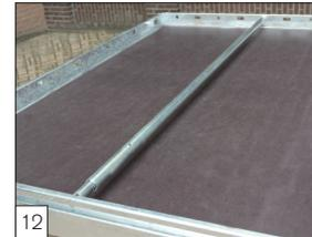
**Option:** load-restraint tubing mounted.
