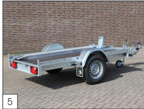
**Standard:** rear lights are integrated in the light girder.
