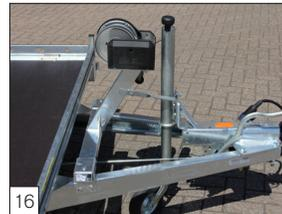
**Option:** winch and winch support mounted in front (only possible on braked versions).
